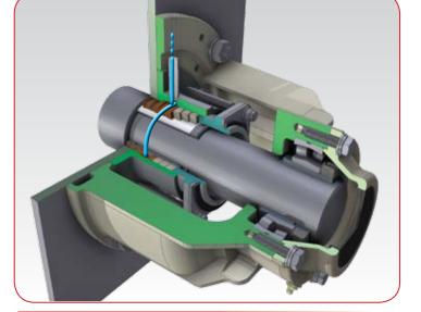
SECTION OF SHAFT AND SEAL
